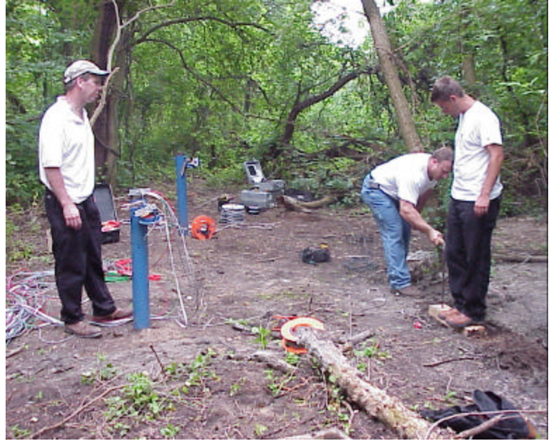
Above: MRCE engineers perform downhole seismic logging of a 250 ft. deep boring on Brooklyn's Shore Parkway for a replacement bridge design.
