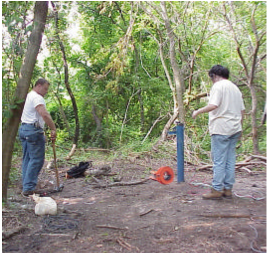
Above: MRCE engineers perform downhole seismic logging of a 250 ft. deep boring on Brooklyn's Shore Parkway for a replacement bridge design.
